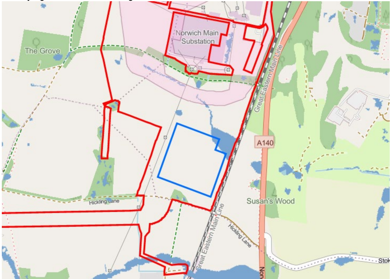
Plate 3-12: Preferred Substation Footprint (Royal Blue Boundary) Taken Forward for the DCO Application. Areas of Potential Surface Water Flood Risk Associated with Naturally Low Lying Areas Shown as Lighter Blue Areas
